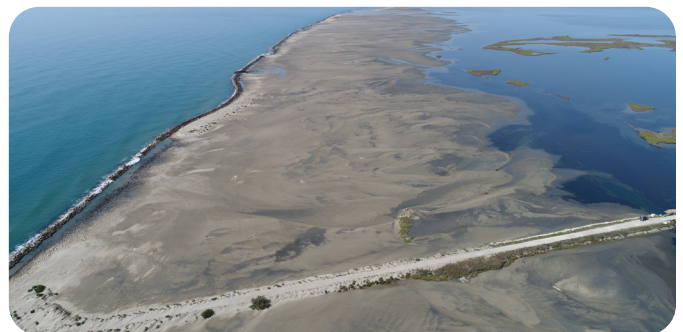
Illustration of the appearance of new beach areas in the south of the buffer area, due to overwash processes in the context of non-maintenance of the historic sea-dikes protection. Mediterranean Sea – left, lagoons – right. © Willm and Arnaud, Tour du Valat.
