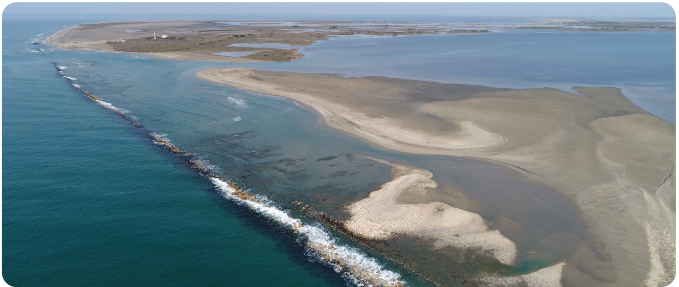
Illustration of the restoration of the natural coastal dynamics in the south of the buffer area, due to the non-maintenance of the historic sea-dikes protection. Mediterranean Sea – left, lagoons – right. © Willm and Arnaud, Tour du Valat.
