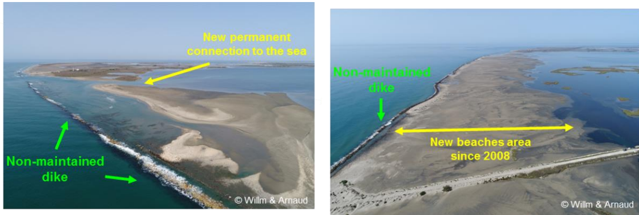
Figure 5.2.4: Aerial drone views highlighting the geomorphological dynamics observed in the southern part of the Rhone Delta Fellow Pilot with the non-maintenance of sea-dikes protection of the former salt production site. To the left: formation of new connections to the sea. To the right: creation of beaches areas. On both views the sea is on the left and the Fellow Pilot is on the right.
