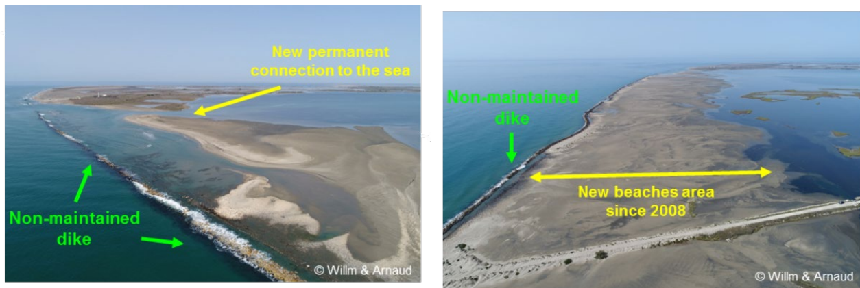
Figure 5.5. Aerial drone views highlighting the geomorphological dynamics observed in the southern part of the Rhone Delta Fellow Pilot with the non-maintenance of sea-dikes protection of the former salt production site. To the left: formation of new connections to the sea. To the right: creation of beaches areas. On both views the sea is on the left and the Fellow Pilot is on the right.
