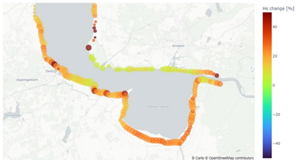
Figure 3.14. Changes in maximum wave height during storm Xaver compared to the same storm event simulated without sea-level rise and changes in ecotopes for the years A) 2030, B) 2050, and C) 2100 in climate scenario ssp 585. The color represents the change as % compared to 2020. The size of each dot represents the associated wave height.
