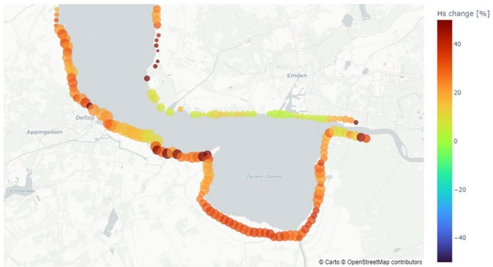
Figure 3.13. Changes in maximum wave height during storm Herwart compared to the same storm event simulated without sea-level rise and changes in ecotopes for the years A) 2030, B) 2050, and C) 2100 in climate scenario ssp 585. The color represents the change as % compared to 2020. The size of each dot represents the associated wave height.
