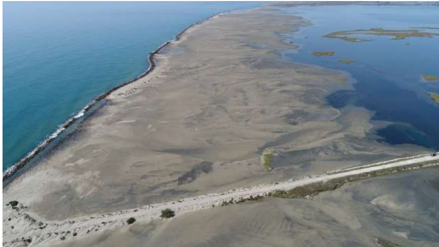
Figure 70 New beach area due to overwash process due to non-maintenance of outer dike (Willm & Béchet, 2023)
