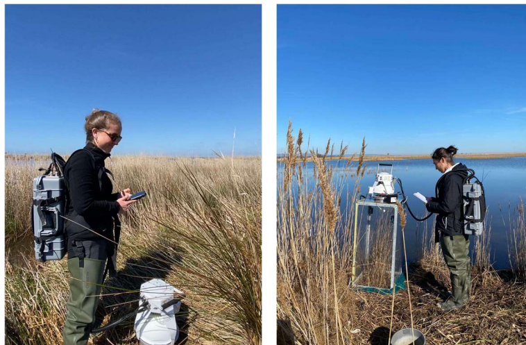
Figure 11. Sampling soil and plant GHG fluxes in the Alfacada lagoon.
