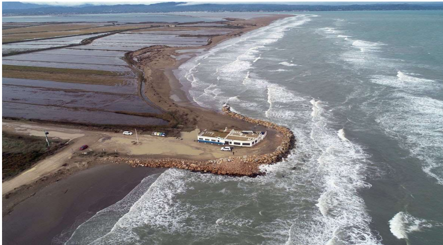
Figure 2. Example of shoreline retreat due to erosion, and hard engineering solution to protect a coastal asset (Vascos restaurant), at the northern end of La Marquesa beach (credit Taula de Consens - Aguaita.cat).
