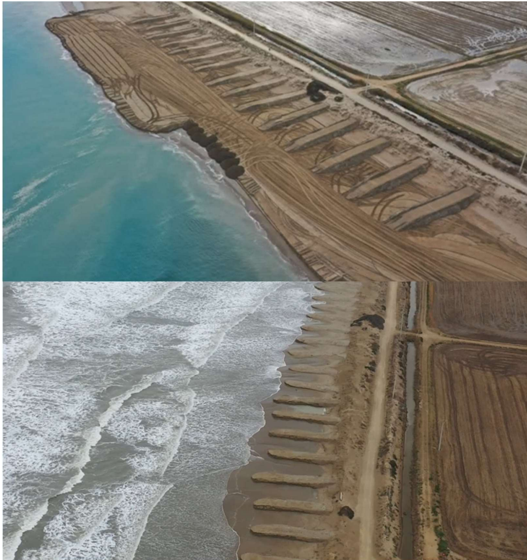
Figure 4. Creation of artificial dunes at La Marquesa beach (top) and state of the dunes after a storm (bottom).
