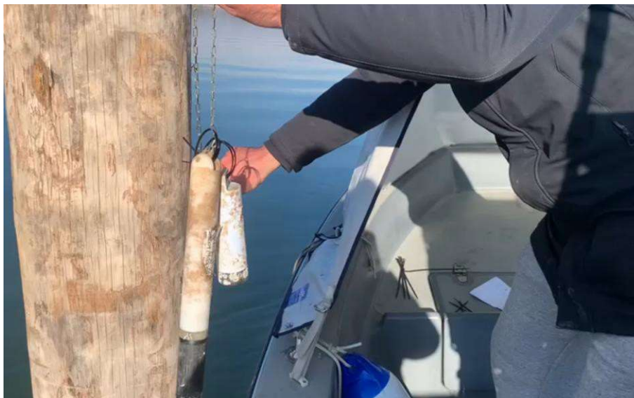
Figure 10: The positioning of the probes for measuring dissolved oxygen and turbidity.
