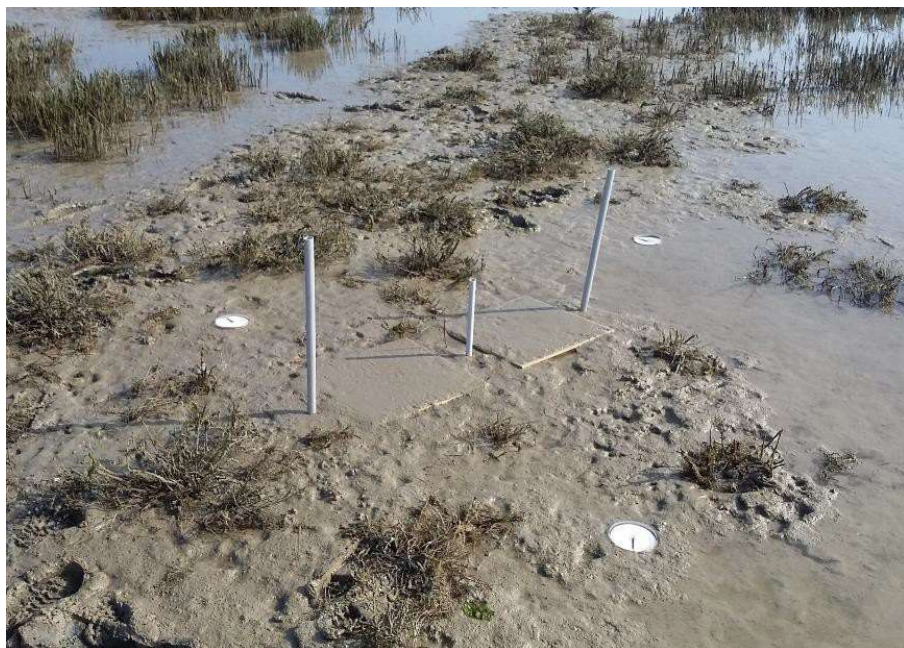
Figure 8: Sedimentation field activities: compaction measurement plates (about one month after installation); Petri dishes for deposition measurement are also visible.
