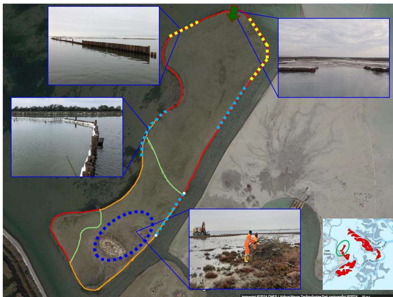
Figure 23: Map of the “Lago della Pietra” saltmarsh, detailing the types of structures and measures implemented: reconstruction of the perimeter piles using 2 different technical schemes (red and orange lines); construction of new embankments within the mudflat surface (green lines), to delimitate the two areas to be filled with new sediments; eradication of shrub vegetation in the higher areas (blue dots); use of geotextile composed of natural fibres (light blue dots); higher piles in order to ensure accessibility for birdlife even during high tide conditions (yellow dots).
