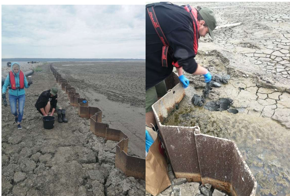
Figure 7 Preparation for (left) and collection of samples (right): very soft condition of soil is clearly visible
