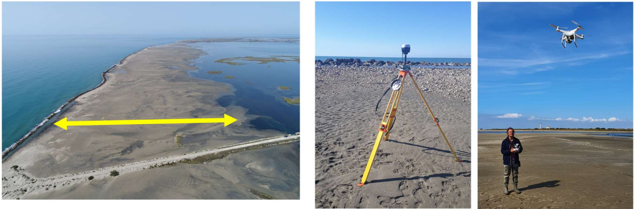
Figure 26: illustration of topo-bathymetry measurements of beach areas, and of the natural channels connecting the site to the sea.
