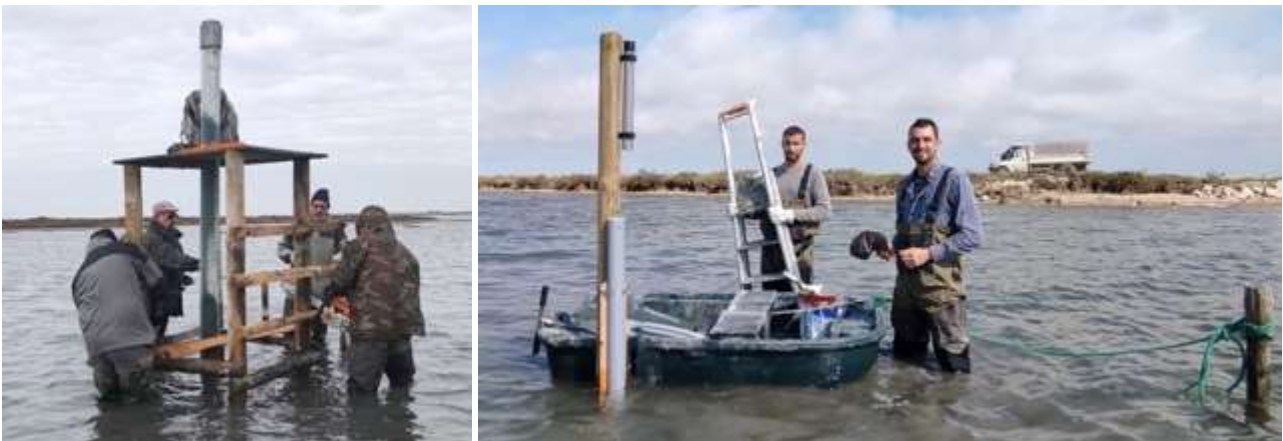
Figure 28: Installation of sensors for continuous measurement of water level, temperature and salinity. Installation carried out in collaboration with the Camargue Regional Nature Park.
