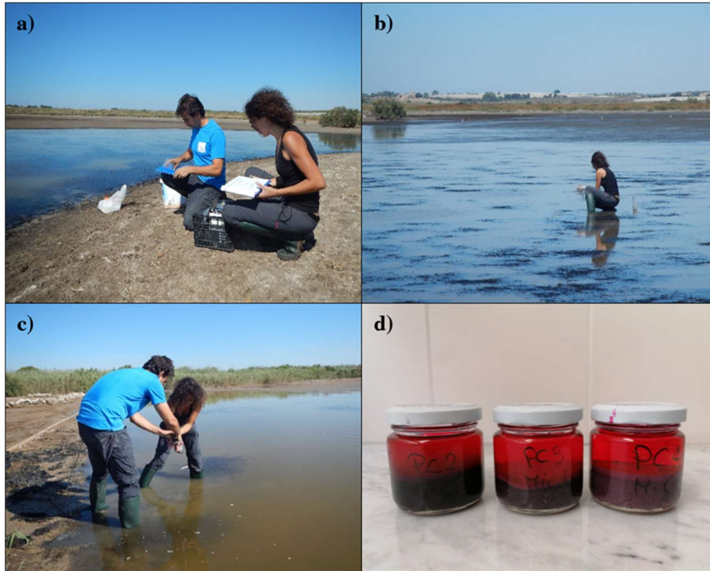
Figure 15: Sedimentological and benthonic surveys operation. a) Labelling of the polythene bags and jar to store the samples; b) Performing sedimentological and benthonic sampling; c) Washing and sieving the microbenthonic sample; d) Microbenthonic samples mixed with Rose Bengal and ethanol solution.
