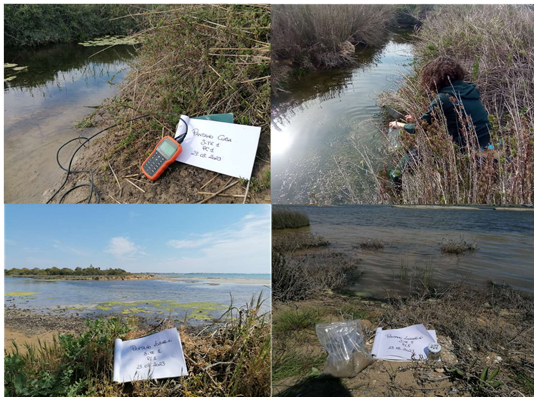
Figure 14: Sediment sampling surveys at the lagoons. Each sampling station has its site name and acronym, coordinates and the date of the survey are also noted. For each site, three sediment samples were collected for grain-size, micro- and macrobenthic analyses.
