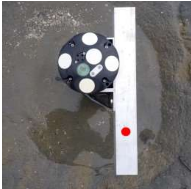
FIGURE 14. REFERENCE POINT TO CALIBRATE VERTICALLY PRESSURE SENSOR AND ADCP. AND
