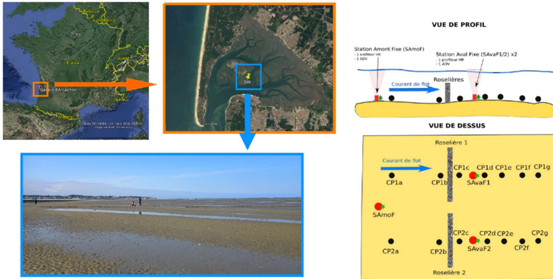
FIGURE 13. LOCATION AND SCHEMATIC PROTOCOL FOR HYDRODYNAMIC SURVEYS TO CALIBRATE ROSELIÈRE DEVICE
