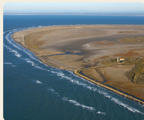
FIGURE 15. BEFORE-AND-AFTER RESTORATION AERIAL VIEW AT THE RHONE DELTA PILOT SITE. IMAGES SHOW THE ABANDONMENT AND GRADUAL COLLAPSE OF THE SEAFRONT DIKE, CREATING A NEW INLET CONNECTING THE SEA TO THE LAGOON. © MICHEL GAUTHIER-CLERC (2011) AND LOÏC WILLM (2024)
